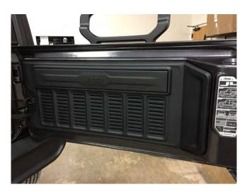
**STEP 2 //** Using a trim panel removal tool, carefully pry the plastic tailgate cover off. Remove cover.
