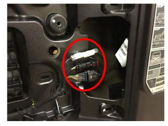
**STEP 3 //** Locate, and unplug the (3) wire connections.
