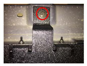
**STEP 6 //**Once the Rubi Rails are tight to the pinch welds, install the (3) M8 x 35mm bolts, flat washers, and lock washers through the body mount brackets.
