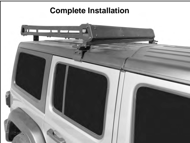
(Fig 16) Front Cross Bar attached to the Front Brackets (passenger side illustrated)
