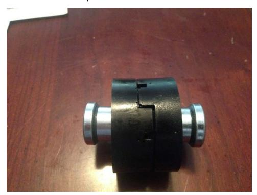
3. Install threaded ring and tighten using supplied spanner wrench. It may be helpful to apply a small amount of grease onto threads before installation. Once tightened, ensure that one of the grooves in the threaded ring is aligned with the set-screw hole.
