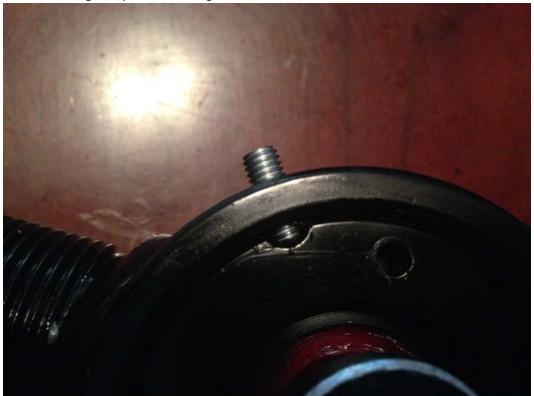
5. Install grease fitting into flex joint housing. Tighten using 3/8" wrench.
