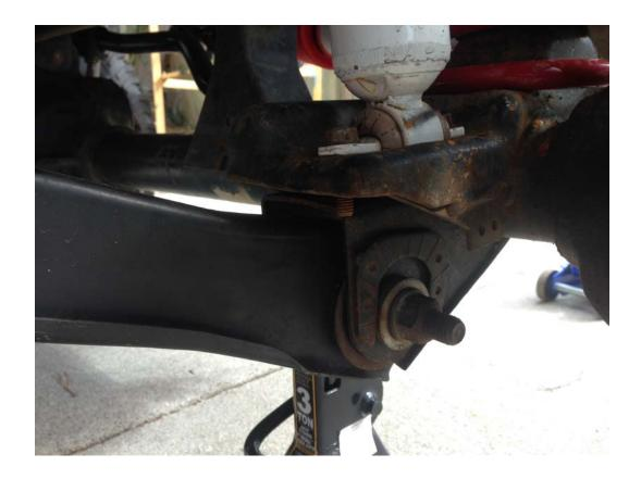
9. Using a tape measure, measure the length of the stock control arm. This measurement should be taken from the center of each eyelet in the control arm as shown in the picture below.
