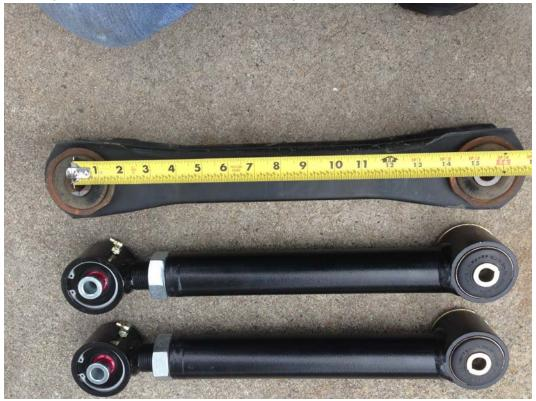
10. Adjust new control arms to desired length by threading the flex joint into the arm. The length of the arm will vary, depending on your vehicle's suspension components, but the stock length is a good starting point. Once desired length is achieved, tighten jam nut using a large adjustable wrench. Ensure that the arm is straight when tightening, by holding the arm on a level surface while turning jam nut.
