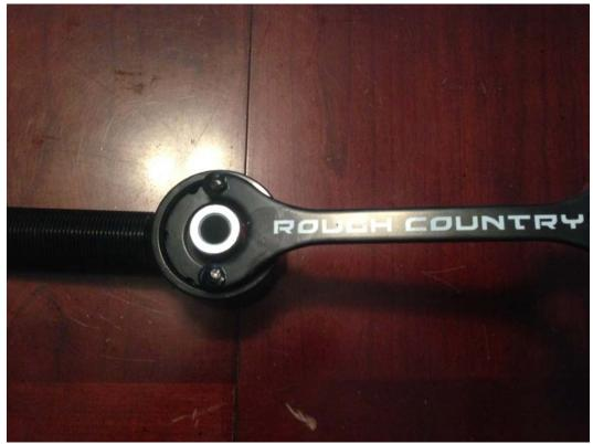
4. Insert set-screw into outer hole on housing end as shown in next photo. Tighten with 3/32" allen wrench. This locks the threaded ring into place, ensuring that it does not come loose over time.
