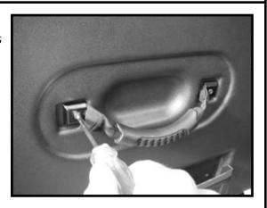
6. Install doors by aligning the door hinge to the holes of the vehicle hinges. Do not force the alignment. It may be necessary to carefully swing the door back and forth several times to allow the hinges to properly seat. Install torx nuts removed in step 3. Tighten to 7 ft-lbs. **NOTICE!** Do not attempt to close door before making adjustments detailed in the next step.
