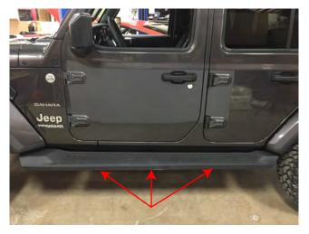
**STEP 1 //** Begin by locating the (3) pinch weld mounting locations under the vehicle.
