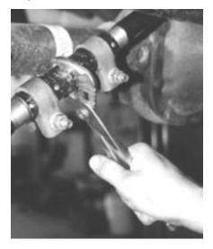
3. Adjust track bar to center the axle under the vehicle. Use the threaded center section and a wrench to lengthen or shorten the track bar.
