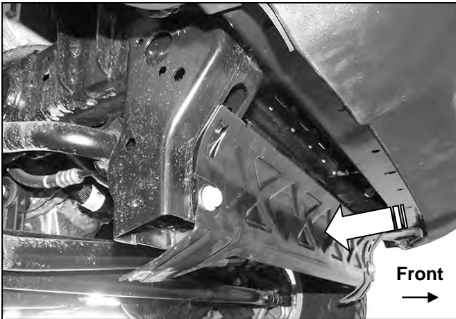
(Fig 1) Remove splash guard and bracket (arrow)
