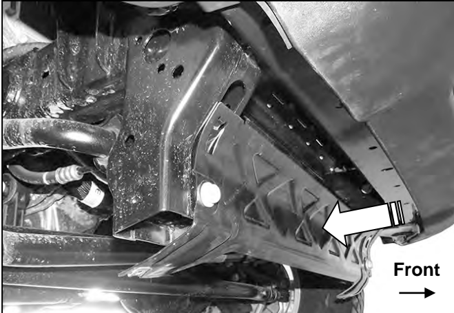
(Fig 1) Remove splash guard and bracket (arrow)
