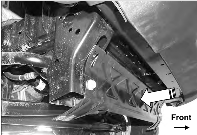
(Fig 1) Remove splash guard and bracket (arrow)
