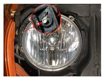
**Step 7:** Headlight Adjustment: Using a T15 torx bit, turn the adjuster clockwise to adjust the light up. Turn the adjuster counter-clockwise to adjust the light down.
