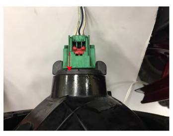
**Step 6:** Plug the headlight harness into the LED light. Push in the red clip to lock harness in place.
