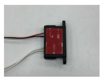
**Step 5:**Mount the resistor to the frame using the supplied adhesive. \*\*Note: The resistor will get hot. Keep away from anything that may cause damage.
