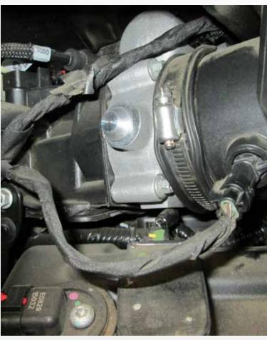
Re-install throttle body control plug, air temperature plug and intake tube back on to BBK throttle body.
