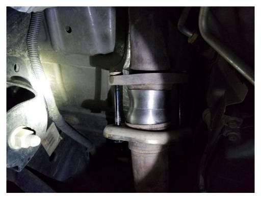
9. Last, retighten the midpipe connector and any other exhaust parts you loosened.
