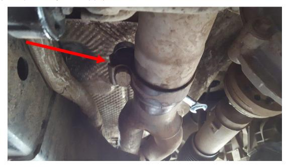
2. Next use a dremmel with a metal cutoff wheel, or a sawzall to remove the small index tab from the Y pipe. Take your time and grind it smooth, it is a tight spot and hard to work in.
