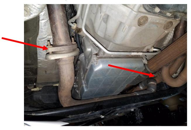
5. The top bolt on the left hand joint is hard to get to, I recommend using a long socket extension as shown below. Once all 4 bolts have been completely removed you can pull apart the 2 joints. You may need to pry them apart.
