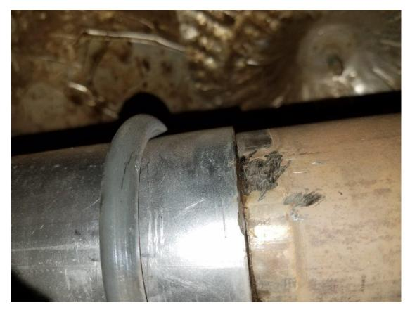
**4.** Using a 13mm socket remove the 4 bolts holding the 2 exhaust joints together. You may need penetrating oil on these bolts to loosen them if your exhaust is older.
