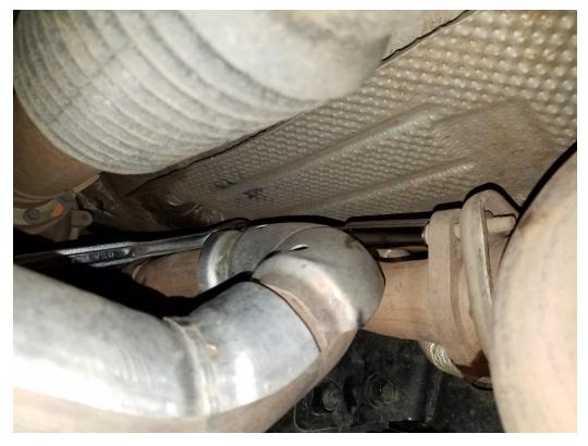
6. Next you will use a pry bar and/or a rubber mallet to slide the Y pipe deeper into the mid pipe. This is why you needed to remove the index tab. This will probably be the most difficult part, depending on the age of your exhaust. I recommend lots of penetrating oil in the pipe joint. This would be easiest if you have a lift and another person to help push on the mid pipe.
