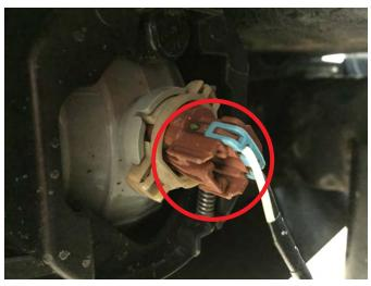
**Step 1\\**Access the connectors on the rear of the fog lights from the wheel well, and remove. \*\*Note: Light connector will be different between 07-09 and 10-18.
