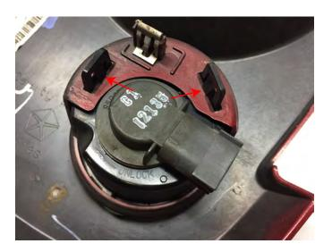
**Step 3**\\ Remove the factory turn signals by unclipping them from the factory grille.
