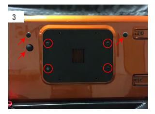
Install the Spare Tire Delete back plate by loosely installing the factory bolts in the holes circled above. Install the (2) small grommets in the factory spare tire bumper mount locations, and the large grommet where you disconnected the factory 3rd brake light.
