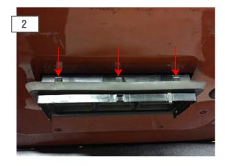
Once the factory mount is out of the way, use a small screw driver or panel removal tool to apply downward pressure the on the tabs highlighted above. To remove, push down and pull the vent off the vehicle.
