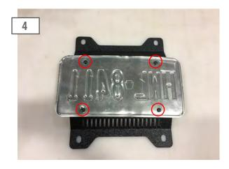
Install your license plate on the outer bracket off the car for ease of installation. Use the (4) Allen head bolts, washers and lock nuts included. \*\*Note: License plate is installed backward for photo purposes only.
