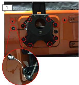
Start by removing the spare tire. Remove the rubber spare tire bumpers. Remove the 3rd brake light grommet from the vehicle and unclip the plug. Remove the (8) bolts holding the factory spare tire mount to the vehicle.
