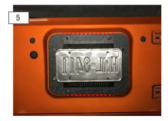
Install the license plate bracket on top of the back plate. With the bolts loose, align the brackets so that they are flush with each other on the top and bottom. Then tighten all bolts.
