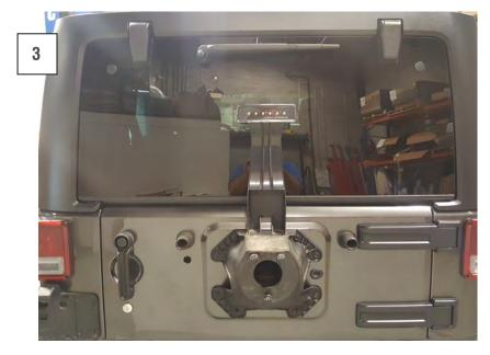
Install the (4) factory screws to the new third brake light.
