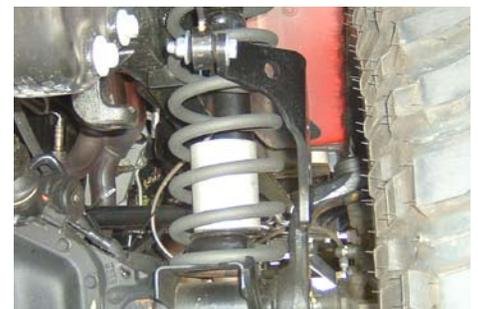
5. Secure the sway bar link to the sway bar mount.
