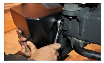
9. If you installed the OE fog lamps into the Brawler bumper, plug the harness connectors back into the sockets in the back of each lamp. Use the OE wire harness pushin retainers to secure the harness to the three (3) provided holes on a flange at the inside rear of the Brawler Lite bumper. You may have to locate them by feel as the area is hard to see once the bumper is installed.
