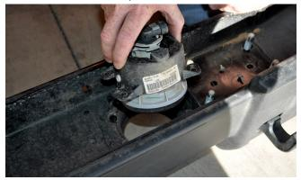
Install the factory fog lamps into the fog lamp mounts in the back side of the Brawler<sup>™</sup> Front bumper. Re-use the OE retaining screws. These sheetmetal screws will form their own threads as you drive them into the retaining rings on the Brawler bumper, so press firmly as you twist the screwdriver.
