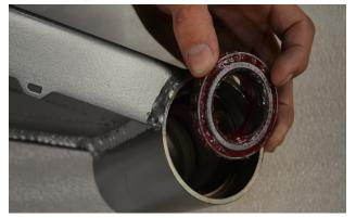
**18. Use a bearing seal driver** tool to carefully install the grease seal into the bottom of the hinge housing. If the proper tool is not available, the step may be performed by carefully using a large socket of the approximate diameter of the seal and a soft dead-blow hammer to work the seal into its seat. Be very careful to drive the seal in evenly, do not let it get misaligned while driving it in.
