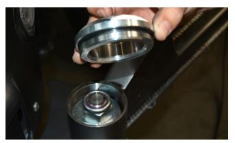
**23. Thread the Hinge Cap onto** the Hinge Housing and <u>lightly</u> tighten with the provided Pivot Cap Wrench. Note that you may have to remove it in later steps to further tighten the spindle lock nut, so don't fully tighten the cap until installation is complete.
