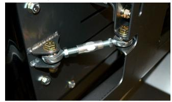
**29. Leave the jam nuts on** the turnbuckle loose, and adjust the length of the tie rod by rotating the turnbuckle. Adjust the length so that the V-Alginment Plate just begins to touch the V-Alignment Bushing when the tailgate is about 1/2" from being fully closed and latched. This is approximately the point at which the tailgate begins to compress the
