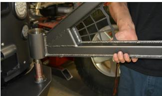
**20. Install the remaining Tapered Roller** Bearing by dropping it down over the hinge spindle, narrow end pointed downward. Carefully slide it down the spindle until it is seated into the upper race.
