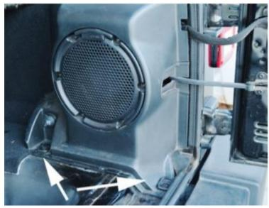
vi. Pull the carpet back behind the roll bar to expose the wiring harness running along the edge of the Jeep's tub.
