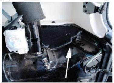
vii. Look closely where the tail lights enter the tub through a rubber grommet. There is a white wire with a purple stripe on it. This is the wire that supplies power to the tail lights and should be used to power a license plate light.
