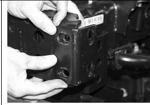
Fig 2 Note the orientation of the bolt holes
