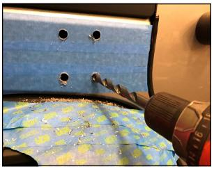
**Step 11:** Install the **10mm** nutsert into the previously drilled **1/2**" holes in the body of the vehicle.
