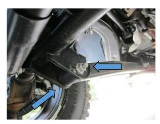
Step Two: Install Skid Plate onto LCA Bracket
