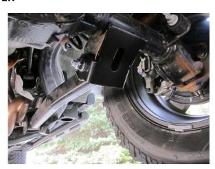
**CAUTION:** As with all steering and suspension components. After driving for a few hundred miles, be sure to re-inspect bolts, and re-tighten to 130 ft. lbs. if necessary.
