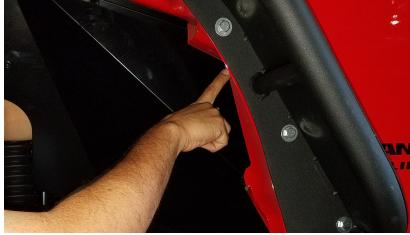
5) You will secure the arm with the supplied longer stainless screw thru the hole in the liner. Tighten the arm while holding it in place. The arm will be at an angle. You can let go of the arm when it is tight enough for it not to drop down. Tighten enough to hold liner secure.
