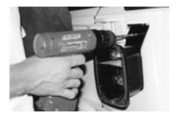
5. Locate the hole in the bracket directly above the tail light housing. Use a 1/4" bit to drill a hole through that hole and through the body. Use the
