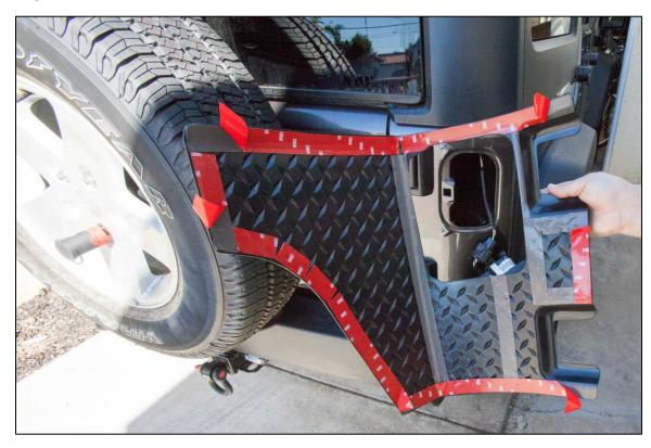
6. Feed the brake light through the corner guard opening and reposition the corner guard near the Jeep body without letting the exposed tape touch the Jeep.
