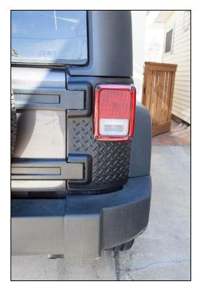
9. Move to the driver's side rear corner. Remove license plate using a flat head screwdriver or 3/8" socket and socket wrench. Remove four license plate frame bolts using a 7 mm socket, extension bar, and socket wrench.
