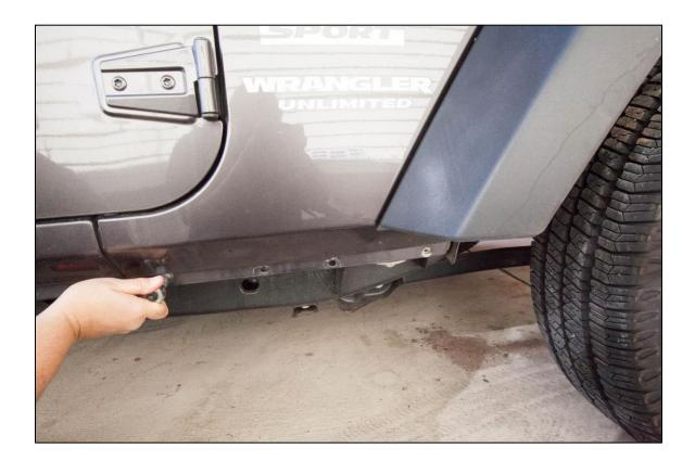
2. Wash, dry, and alcohol wipe the pinch seam and rocker panel.
