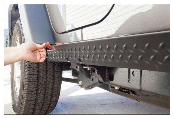
9. If supplied clip fits around rocker guard and Jeep body, attach supplied clip to rear corner of rocker guard. Otherwise, discard clip.
