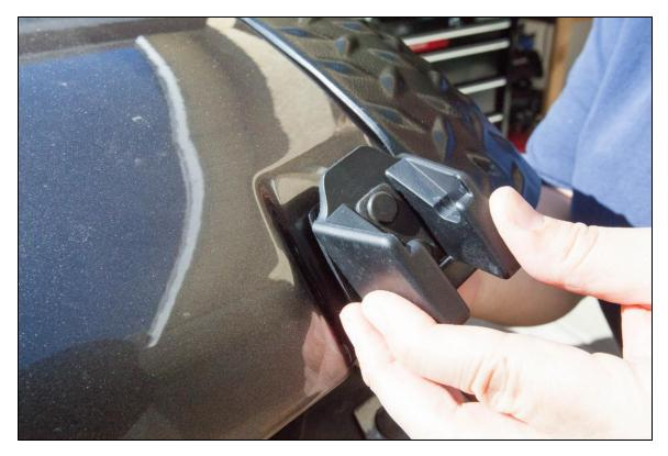
6. Remove protective covering from tape, using previously created grab handles, while pressing hood armor firmly into place as tape is exposed.
