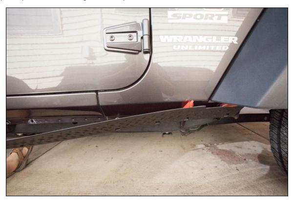
4. Peel two inches of protective covering away from tape. Bend covering up and away to create a grab handle. Align front edge of rocker guard with front edge of frame (near front passenger's side tire). Lightly press exposed tape section against Jeep body to temporarily hold in place while attaching hardware.
