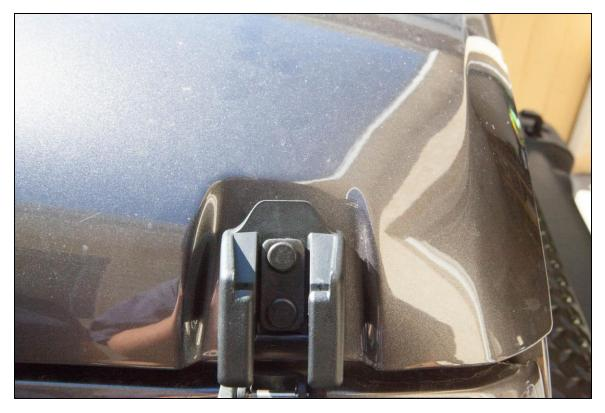
2. Using a 1/2" socket and socket wrench, remove the upper hood latch bolts from the inside of the hood. The lower hood latch bolts do not need to be removed from the body of the Jeep.
