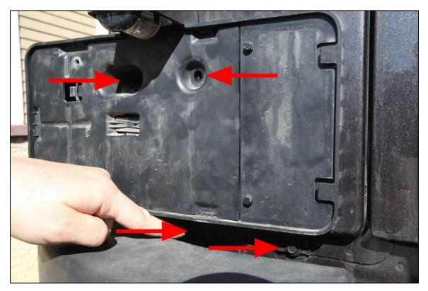
10. Using a flat head screwdriver, gently release license plate lighting wire from capture bracket and disconnect wiring harness.
