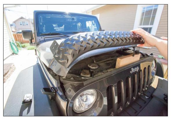
Peel two inches of protective covering away from tape. Bend covering up and away to create a grab handle. Align the hood armor bolt holes with the hood latch bolt holes and loosely install your hood latches using a 1/2" socket and socket wrench.
