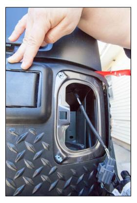
8. Reinsert and reattach the tail light using factory screws and a Phillips head screwdriver.
