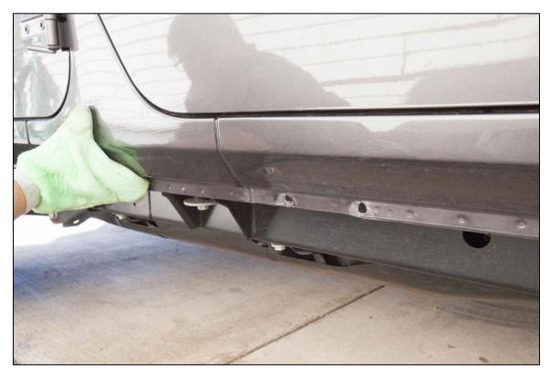
3. Dry fit the rocker guard, making sure the rocker guard bolt holes line up with the factory pinch seam bolt holes. You may need to widen the rocker guard bolt holes if they don't align with the pinch seam bolt holes. Also, if rocker guard end protrudes into rear tire well, mark rocker guard for trimming. Pull rocker guard away from body of Jeep and trim excess length with utility knife.
