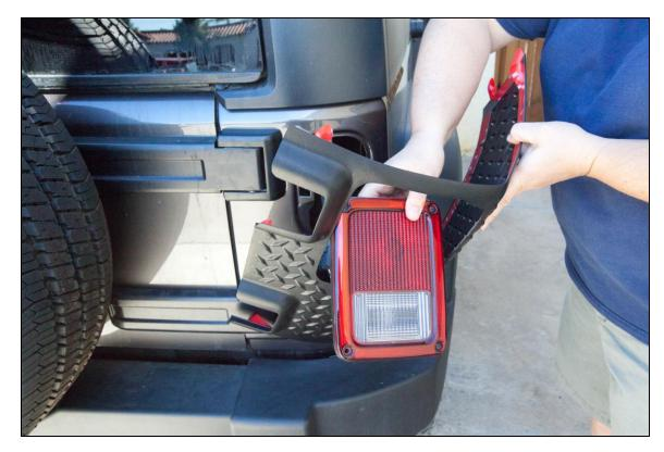
7. Align center of corner guard with corner of Jeep. Press exposed tape section against Jeep body and hold firmly in place while using previously created grab handles to remove remaining protective tape covering.
