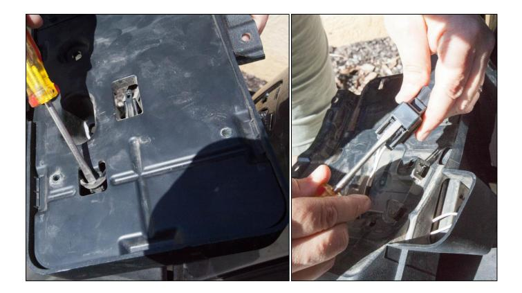
11. Using a Phillips head screwdriver, remove two right-side screws of the driver's side tail light and gently pull the tail light housing away from the body of the Jeep. You do not need to remove the two left-side screws.
