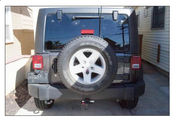
2. Using a Phillips head screwdriver, remove two left-side screws of the passenger's side tail light and gently pull the tail light housing away from the body of the Jeep. You do not need to remove the two right-side screws.
