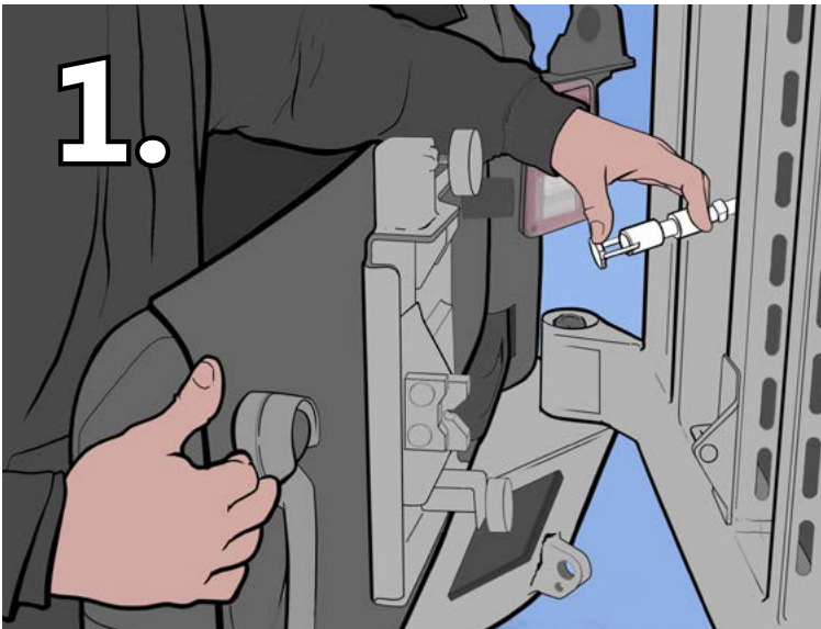
QUICKLATCH + JACKSCREW + BALL STUD
