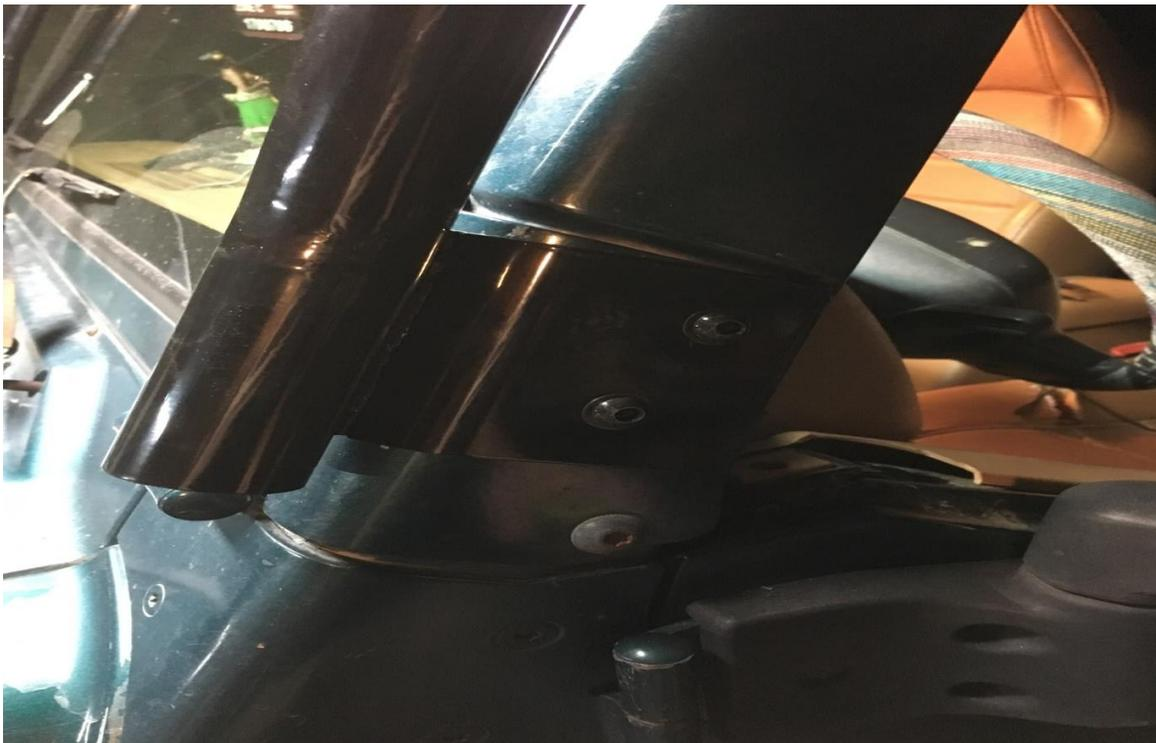
Mount crossbar onto uprights and put Philips screw with washer into hole. Hand tighten
