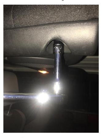
3. Once the screws are out, take one of the screws provided and place the washer through it. Then place the grab handle onto the screw, and finally place the washer taken out in step 2 onto the screw.
