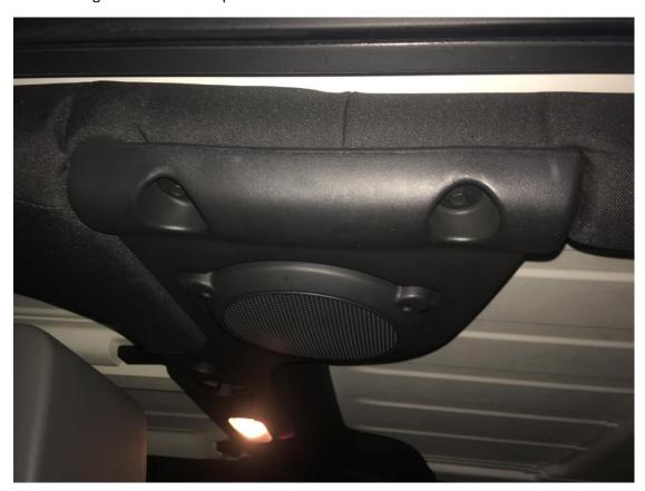
2. Begin by taking removing the two 10mm screws next to the top speaker with a 10mm socket. NOTE: The washer that comes off when you take the screw out will be used again.
