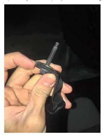
3. Place this in the hole and tighten the screw with the 10mm socket.
