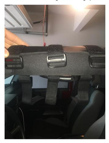
4. Begin to strap the handle with the Velcro straps, starting in the center.
