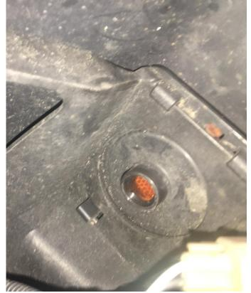
4. Take the side marker out of the fender by sliding it downward toward the ground.
