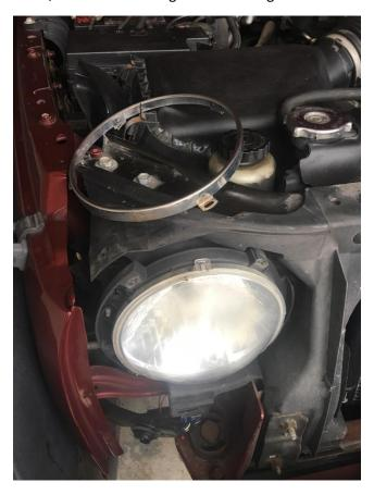
5. Place the light guard onto the headlight, making sure to align the holes of the light guard with the holes on the Jeep. Re-install the screws taken off in step 3.
