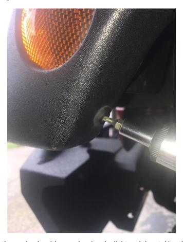
3. Remove the light from the marker by either unplugging the light and then taking the light out, or taking the whole assembly out together. This is the marker with the light taken out.
