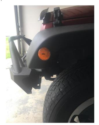
2. Using something long and thin, punch out this thing holding the fender and the inner fender liner together. (I used a T10 Torx bit on my screwdriver.
