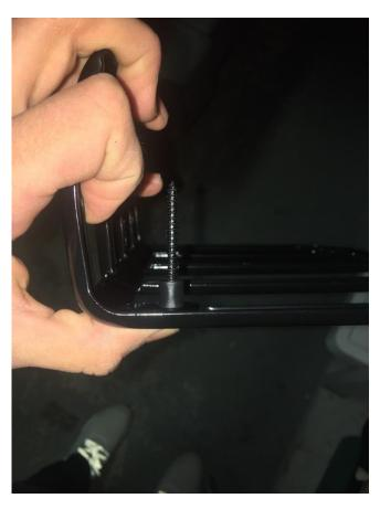
4. Place the guard onto the brake light and slightly tighten the screw. Repeat step 3 until all screws are slightly screwed in.
