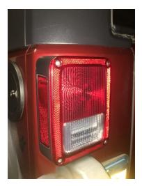
2. You are given 4 screws per brake guard. The larger screws will be placed on the outside of the brake light. (Larger screws are the two on the right side)
