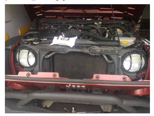
7. Re install the grille, turn signal bulbs and screws that hold the grill in place. Close the hood.
