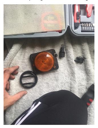
5. Place the guard into the fender, from the inside, and then replace the side marker.
