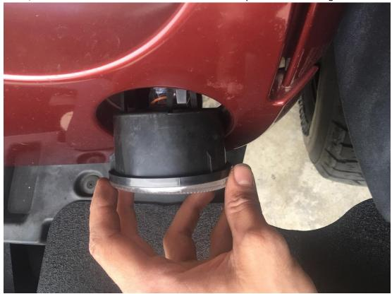
3. Place the guard onto the turn signal by aligning the 3 metal tabs on the guard to the 3 tabs on the turn signal housing. NOTE: This is a very tight fit. You may have to adjust some of the metal tabs manually for it to fit perfectly.
