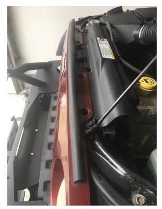
2. Remove the grille by removing the turn signal bulbs and pulling it from the lower retaining clips. (Lower retaining clips are shown behind the grille)
