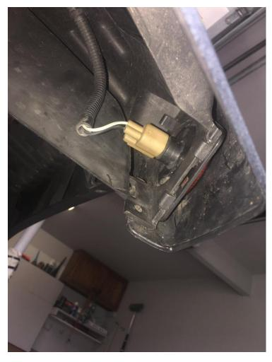
7. Replace the piece that held the fender and inner fender liner together.
