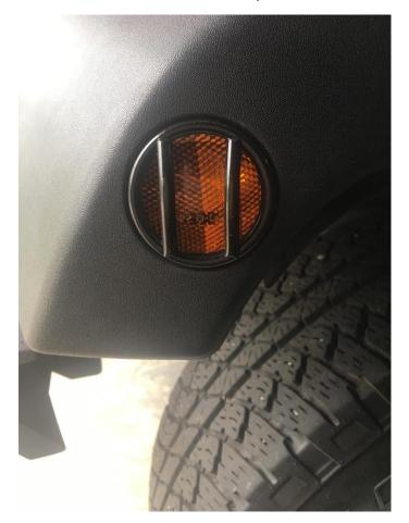
6. Replace the light assembly to the side marker. (View from underneath the fender)
