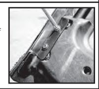
Step 6. With the assistance of a second person, raise the top and bow assembly in the up position. Lock the header to the windshield. Carefully drape the top over the windshield onto the hood. With the top portion of the header exposed remove all of the screws from the top side of the header. Remove the top portion of the header. Remove the old top from the header.
