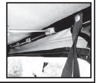
Step 4. Unfasten the hook and loop retainer that secures the top to the bow located above the roll bar. It may be necessary to lower the top at this time to aid in the removal.
