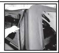
Step 2. Release the rear corners of the top. Pull down and out on the rear corners to remove the fabric from the belt rail. Repeat this procedures for both sides.
