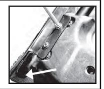
Step 9. With the assistance of a second person, raise the top and bow assembly in the up position. Lock the header to the windshield. With the top laying loosely over the bow assemblies, re-attach the fabric to the bows using the screws removed earlier. The fabric on the rear bow wraps under from the back side of the bow toward the front of the vehicle. The fabric on the middle bow wraps over the top and the front side of the bow.
