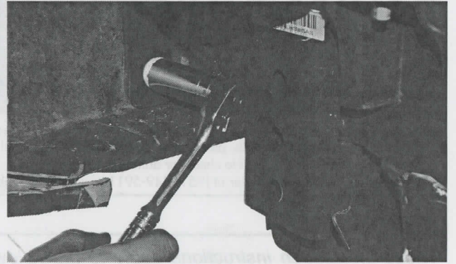
With these nuts removed, remove the bumper from the Jeep.
