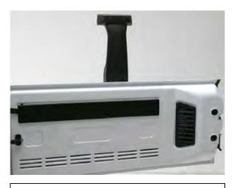
Step 2 Open rear swing gate to access 3<sup>rd</sup> brake light plug
