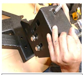
Step 3 Place the tire carrier onto tire carrier arm.
