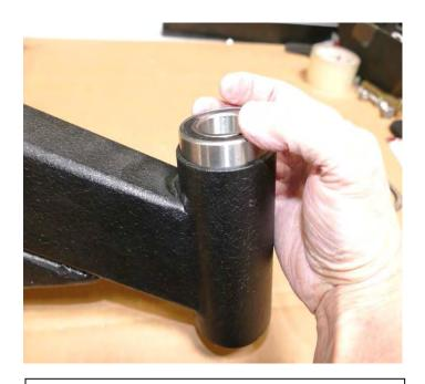
Step 3 **WORKING ON WORK BENCH**Place supplied sealed bearing (N) on the upper side of the tire carrier spindle hub. Carefully center bearing on the spindle hub and tap the bearing into position with a rubber mallet. Be careful to drive the seal evenly and not to damage it.
