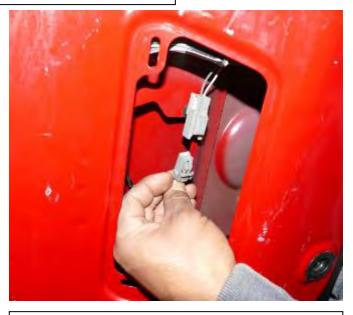
Step 6 Open rear swing gate and connect the brake light. Re-install factory panel cover removed in page 2.
