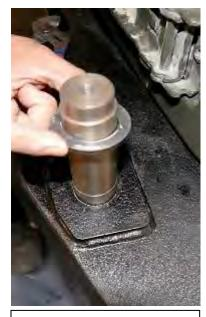
Step 1 Install supplied ring spacer (Y) on bumper spindle.
