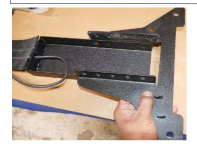
Step 1 **Working on work bench.**Install supplied brake light mounting bracket (L) onto supplied brake light (K) as shown. Line up brake light holes onto mounting bracket.
