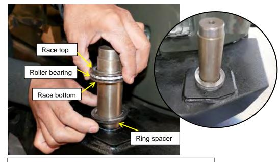
Step 2 Install supplied bearing race, roller bearings, and bearing race onto spindle in that order. Using wheel bearing grease (not supplied) coat the spindle and bearings.
