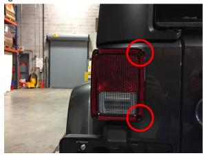
Step 2: Disconnect the tail light plug and then remove the light from the vehicle.
