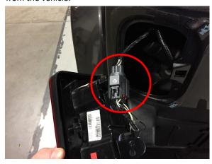
Step 3: Install the resistor to the mounting bracket using the supplied bolts and lock washers. Install the clips on the resistor brackets.
