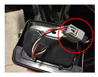
Step 4: Install the LED tail light with the factory screws. Reconnect the battery terminal and ensure the tail light functions properly.
