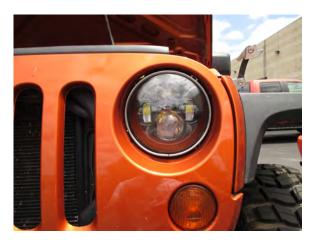
Step 6: Reinstall the headlight bezel and repeat the process in reverse to reinstall the grille.
