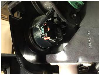
**Step 1\\**Access the connectors on the rear of the turn signals from the wheel well. The turn signal clips have a red locking tab, first slide the locking tab out. Then depress the clip to remove the signal plug.
