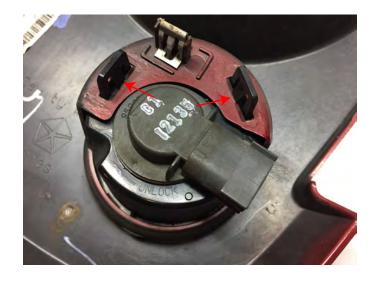
**Step 3\\**Remove the factory turn signals by unclipping them from the factory grille.
