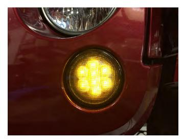
**Step 4\\**Install the new LED turn signal in reverse order.
