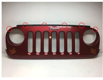
**Step 2\\**Using a panel removal tool, remove the (6) push clips holding the grille cover to the vehicle. Unplug the turn signals and pull the grille cover from the vehicle.
