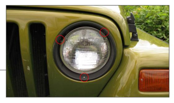
Remove the (3) T15 torx screws that secure the outer trim bezel.
