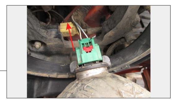
Slide the red retaining clip away from the plug. Then disconnect the plug from the headlight.
