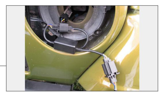
Unplug factory headlight. Connect the LED Headlight using the supplied jumper harness. Firmly press the plugs together and push the retaining clip from the factory harness back into the plug.
