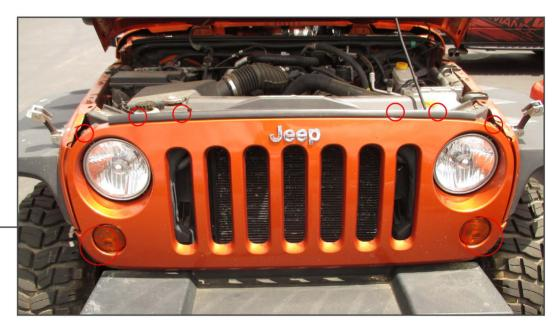
Open Hood and remove the six (6) plastic clips holding the grille to the vehicle. There are clips along the bottom of the grille that snap into the metal radiator support. To release the clips, pull the top of the grille away from the vehicle while gently pulling on the bottom edge. Increase pulling pressure slowly, being careful not to aggressively pull, so you don't damage the clips or scratch the grille. Disconnect the turn signal plugs and remove grille from vehicle.
