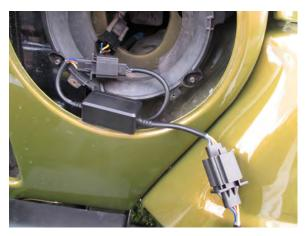
Step 4: Secure wiring components and reinstall the headlight bezel. Reinstall the trim bezel.
