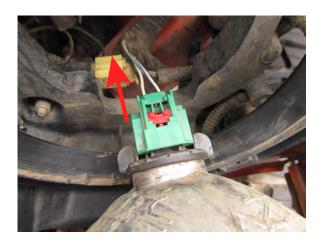
Step 4: Connect the LED Headlight using the supplied jumper harness. \*\*Note: firmly press the plugs together and push the retaining clip from the factory harness back into the plug.
