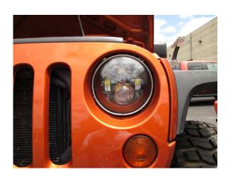
Step 5: Reinstall the headlight bezel and repeat the process in reverse to reinstall the grille.
