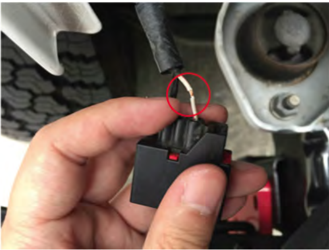
Splice the Green wire from the headlight to the factory turn signal power as seen above.
