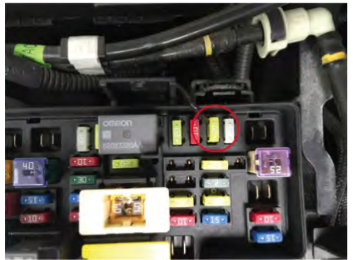
Tap the Red wire from the headlight into the 12v+ ignition wire in the fuse box as seen above.
