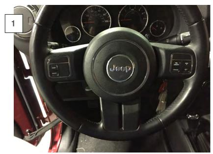
Thoroughly clean the steering wheel, removing any grease/oil contaminants. \*\*Recommended: Wipe the steering wheel trim with isopropyl alcohol to ensure the cleanest surface possible. Allow the steering wheel to dry prior to installing the trim pieces.
