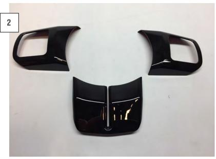
Familiarize yourself with how the trim fits prior to peeling off the double sided tape. Then remove the tape and apply firm even pressure to ensure proper adhesion.
