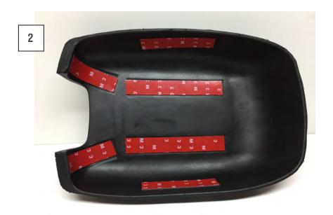
Test fit the arm rest before peeling off the tape backing. Once you are comfortable with how the part should fit, peel off the tape backing.
