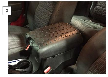
Install the Armrest Cushion, apply firm even pressure to ensure proper adhesion.
