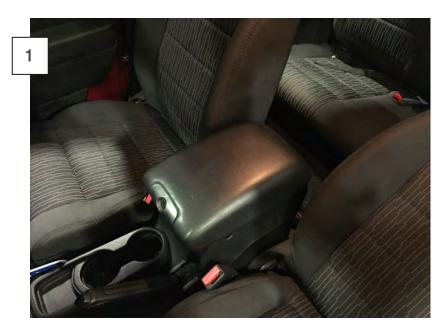
Thorougly clean the center armrest with a silicone free cleaner. Then wipe the armrest down with isopropyl alcohol to ensure the cleanest surface possible.
