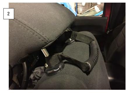
Slide the grab handle ends over the headrest posts. Reinstall the headrests.
