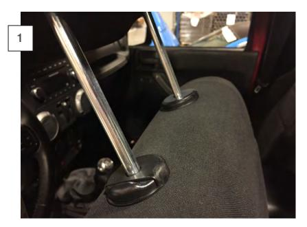
Raise the headrest and depress the inner tab to release the headrest from the seat.
