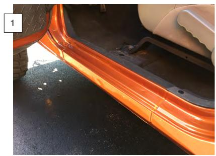
Wash the Door Sills with soap and water. Allow the sills and surrounding areas time to dry. \*\*Recommended: Wipe the sills down with isopropyl alcohol to ensure the cleanest surface possible.
