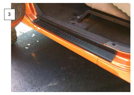
Install the Entry Guards on to the vehicle. Apply firm even pressure to ensure proper adhesion.
