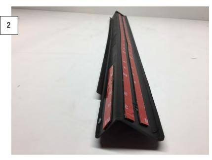
Test fit the Entry Guards to familiarize yourself with how they fit. then remove the 3M tape backing.
