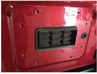
**Step 3\\**Remove the tailgate vent and grommet from the vehicle.
