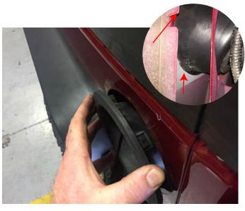
**Step 2\\**Remove the gas cap from the filler neck. Through the tail light opening, use a long flat head screwdriver, depress the (2) visible clips.
