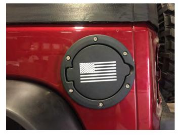
**Step 4\\**Transfer the fuel filler cap to the new housing and then reinstall in reverse order.
