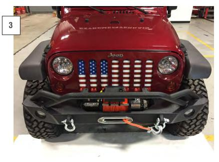
Reinstall the grille, once the insert is centered, reinstall the factory push clips.
