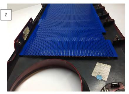
Wedge the insert into the grille cover. It is held in with pressure. Once on the vehicle, center the insert in the grille.
