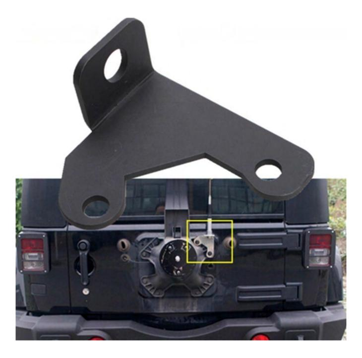
Remove the (2) factory 13mm tire carrier bolts. Reinstall the bolts through the CB Antenna mount.
